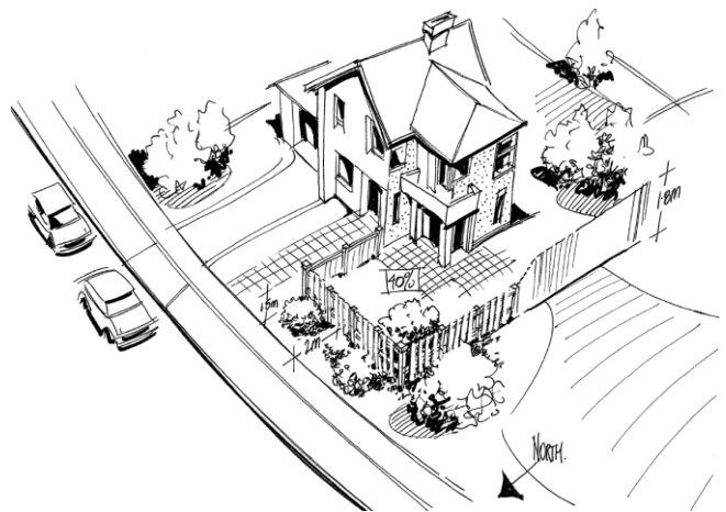
Front fences to north facing front yards
